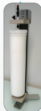
Standalone column holder for flash chromatography
