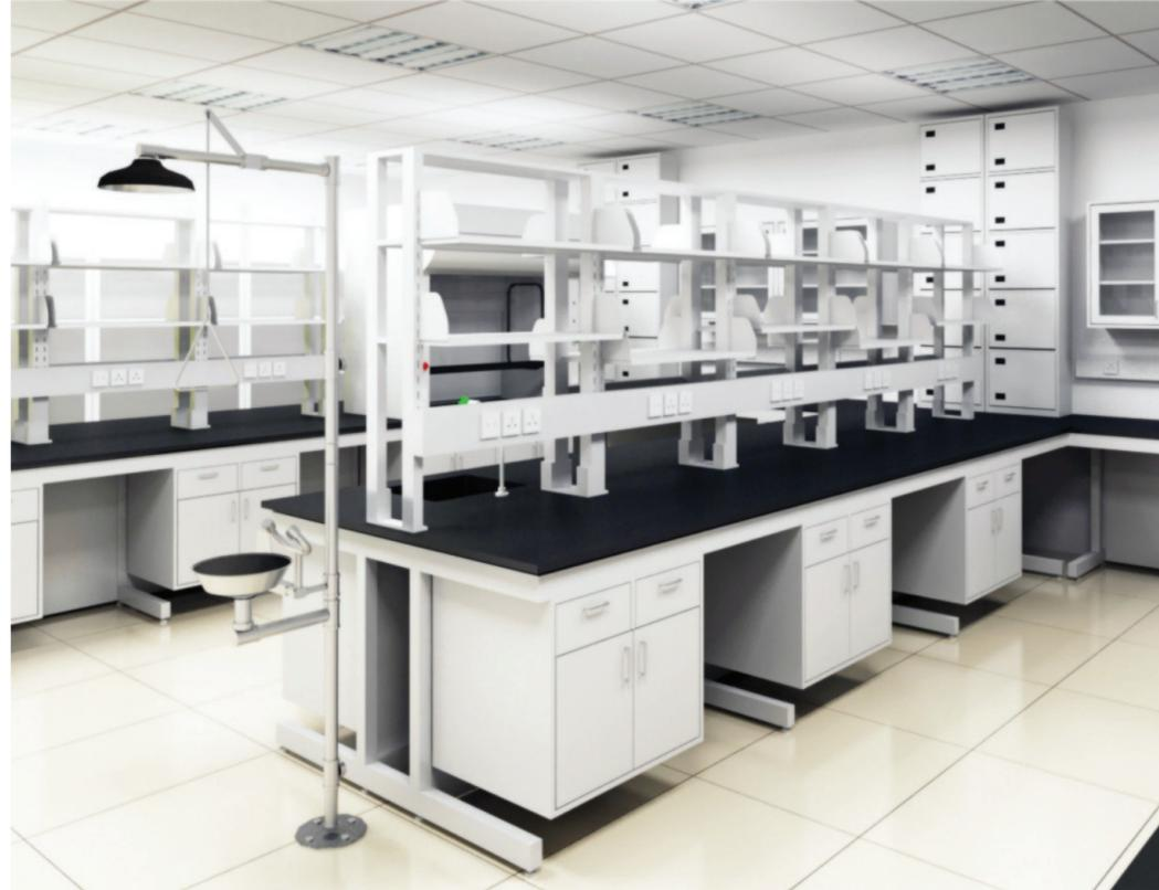
Fisher Scientific's CFrame laboratory furniture system has been a laboratory standard for several decades. The C-shaped frame supports removable upper and lower storage cabinets and work surfaces. Storage cabinets can be positioned at any point horizontally along the table frame, and are easily removed or repositioned for under-counter refrigeration, cart storage or knee space areas.
